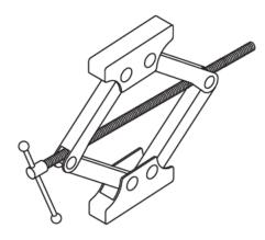
The device is modelled by a rhombus of side length 25 cm.
